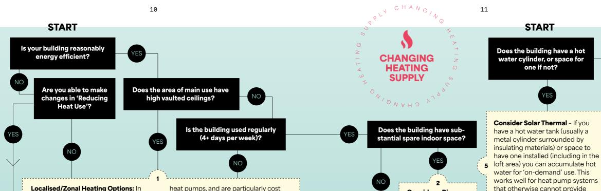
buildings with very high ceilings and/ or poor insulation, it is challenging to provide warmth to people in the building through circulating warm air–as traditional boiler and radiator systems do. Where a building is not in regular use, it might not be cost effective to install new heating that warms the whole building. In these circumstances, localised heating can be more effective to keep people warm.
